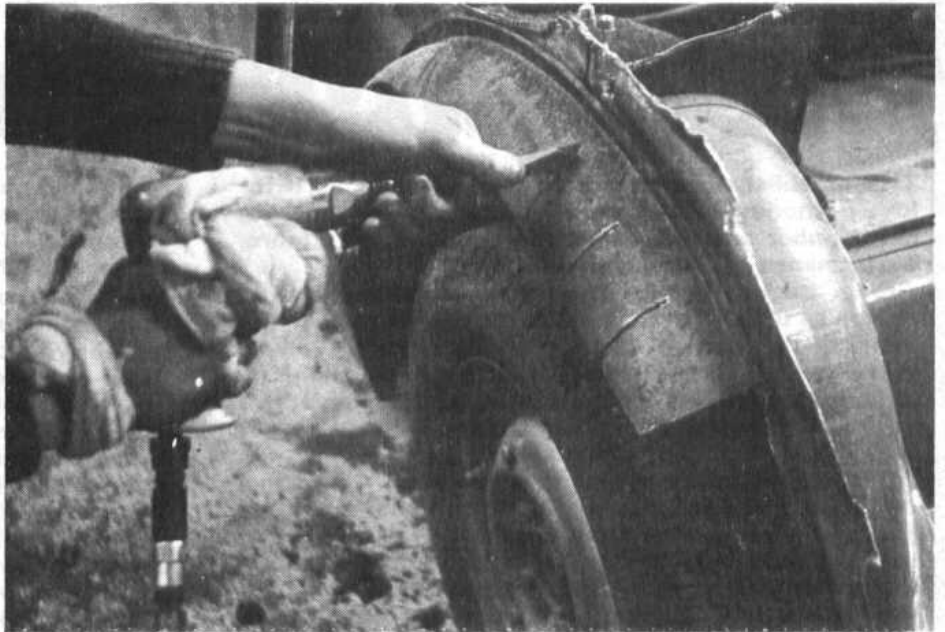
When the arches have been cut back to leave only three inches of metal, cut slots in toward the centre.
