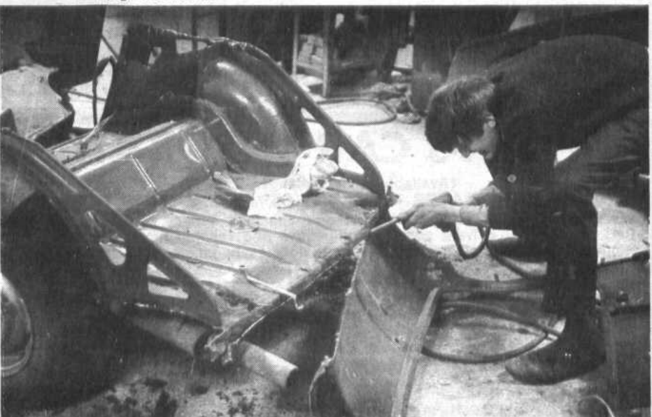
Attack the metal at the top of the support frames on both sides, so that the whole of the central panel can be lifted off... it is best to cut the metal at the back of the floor first.
